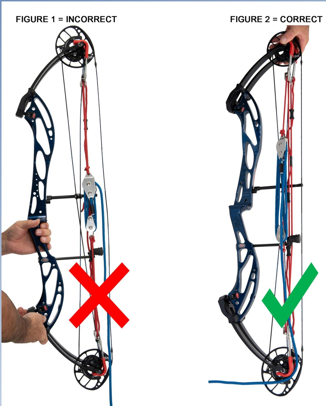
As the red rope has not been adjusted in Figure 1, it will be impossible to press the bow as the blue rope needs more length as shown in Figure 2.
